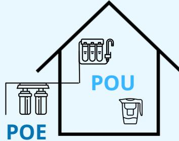
**POU filters** are installed at the tap or are used as pitcher filters. They usually filter water for cooking or drinking.
